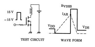
$$\begin{array}{ll} \mathrm{R_{G}=25\ \Omega} \\ \mathrm{V_{DD}=90\ V,\ L=25.5\ mH} \end{array} \quad \quad \mathrm{E_{AS}=\frac{1}{2}\cdot L\cdot I^{2}\cdot \left(\frac{\mathrm{B_{VDSS}}}{\mathrm{B_{VDSS}-V_{DD}}}\right) } \end{array}$$
